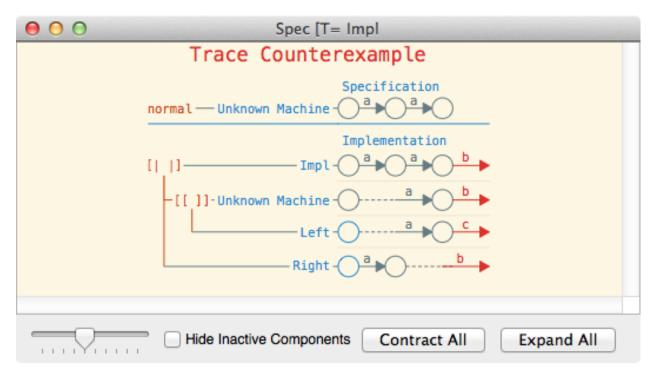
The left portion of the diagram shows the structure of the machines. In particular, we can deduce that the implementation process (i.e. Impl) is a parallel composition of Right and a renaming of Left (the operator arguments can be viewed by *hovering* over the operators themselves).
